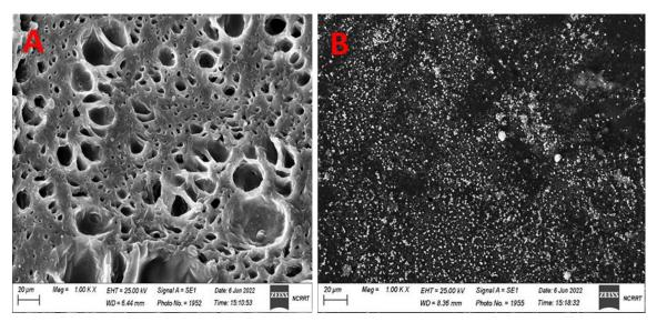
Fig. 1. Photomicrograph of HRTEM measurement, A) Cross section image for cross linked and porous PVA/ Gelatin containing silver nanoparticles after gamma irradiation process at 2.5 kGy, B) Surface mode image for the same sample
