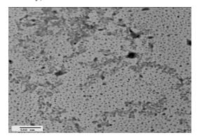
Fig. 3. The TEM image of PVA/PVP/ Ni nanocomposite films (0.015M &170 kGy )
