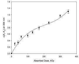
Fig. 4. Change of response as a function of absorbed dose for PVA/PVP/Ni nanocomposites film (0.015 M)
