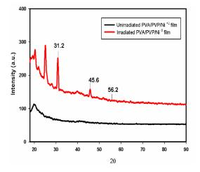
Fig. 2. XRD pattern of the unirradiated and irradiated PVA/PVP/Ni composite films, at 170 kGy
