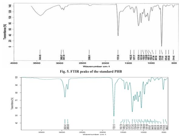
Fig. 6. Infra-Red spectrum of PHB purified product
