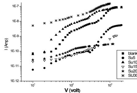
Fig. 1. I – V Characteristic curves for untreated Clay samples at room temperature (300K).
