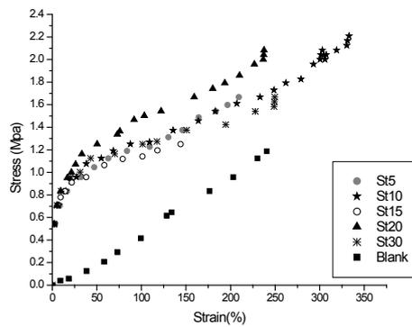
Fig. 6. Stress –strain curves for treated samples at 300K.
