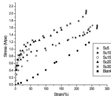
Fig. 5. Stress-strain curves for untreated samples at 300K.
