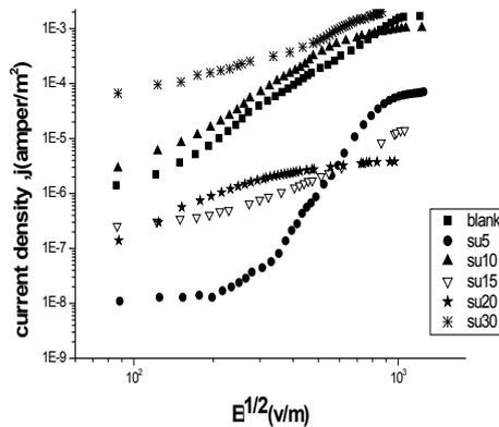
Fig. 4.  $\log(J)$  versus  $E^{1/2}$  for unmodified samples.
