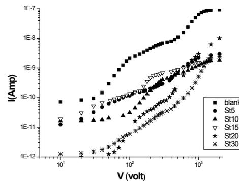
Fig. 2. I – V characteristic curves for treated Clay samples at room temperature (300K).
