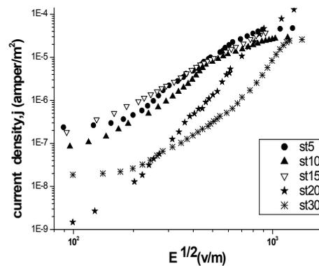
**Fig. 3. Log (J) versus  $E^{1/2}$  for (SMEB) samples**
