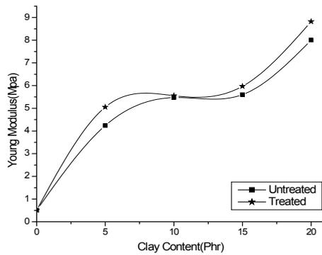
Fig. 8. Young's modulus versus clay loading for untreated and treated samples (at 300K).
